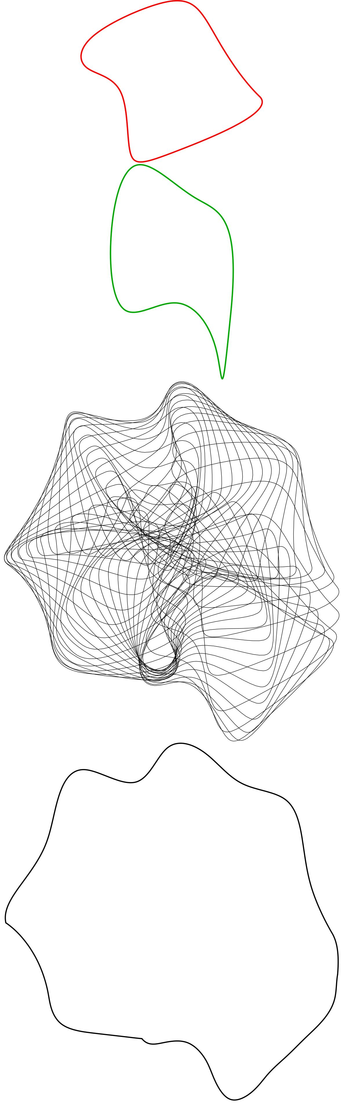
(a) The generator (b) The translation component of motion (c) Generator at a few time instants (d) The boundary of the swept volume.
